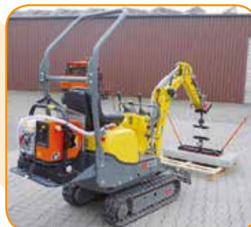
Integrated Vacu-Magnet 500 P at the rear of mini excavator.
