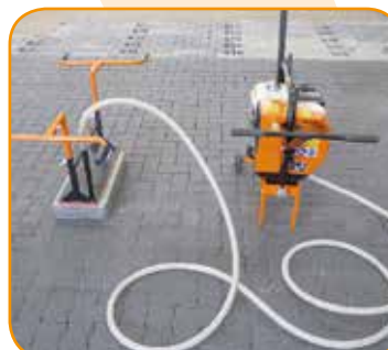
Vacu-Magnet 500 P as vacuum-station.
